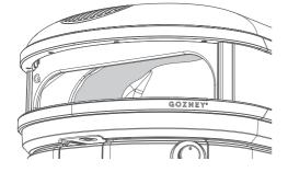
The flame should be yellow in colour and roll along the top of the oven.
