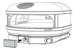
Only when the oven is cold, remove the thermometer and unplug the cable. Gently roll the oven over onto its side and use the torx screwdriver to remove the bottom panel of the oven. Use the spanner to unscrew the old probe from inside the oven and replace it with the new one. Thread the cable back through to the front of the oven and plug it back into the thermometer. Replace the bottom panel and return the oven to its upright position.
